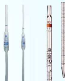
Pipette with Bulb & graduated
